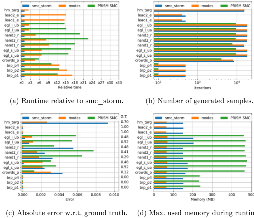
Fig. 1: Performance evaluation of smc_storm , modes , and PRISM SMC (y-axis) on P properties using multi-threading where available. If no bar is present, the test was skipped (20 min limit).
